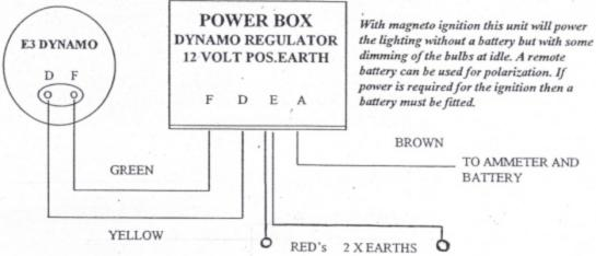
MOUNT IN ANY POSITION, THE LUCAS COVER CAN BE PUSHED OVER THE UNIT AND HELD WITH LOCKING WIRE OR CLEAR PLASTIC STRAP. THIS WILL GIVE AN ORIGINAL APPEARANCE WHEN REQUIRED
