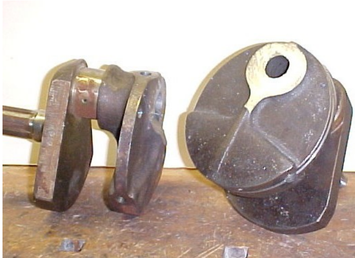
Figure 6 – Donor cranks before machining
