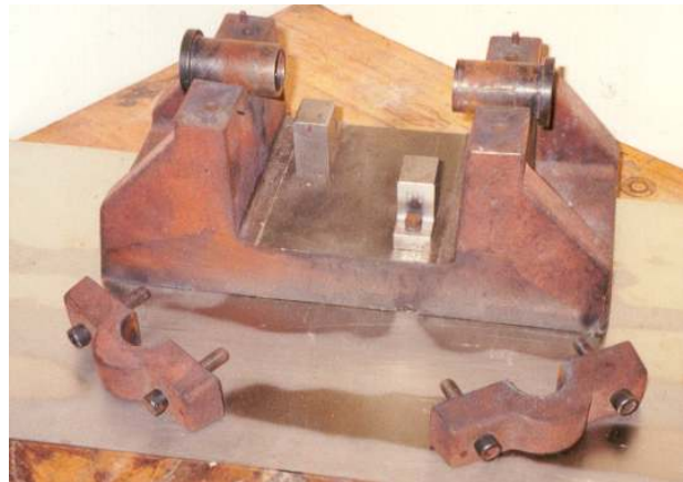
Figure 1 – The fixture with bushings, clamps and stops to position crank throws.
