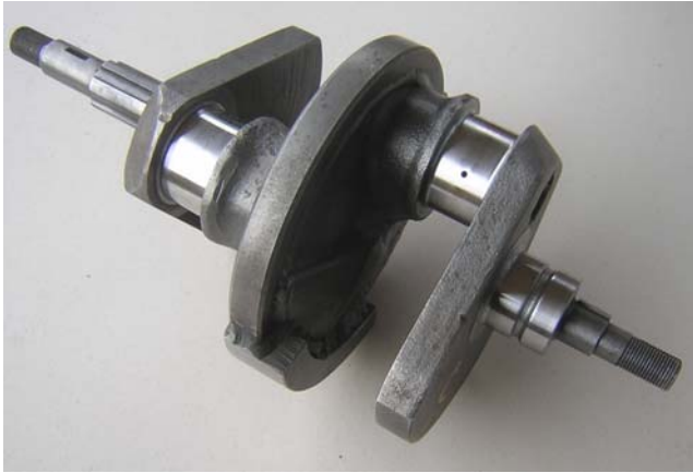
Figure 9 – BSA A65 crank, 16 pounds and 6" in diameter
