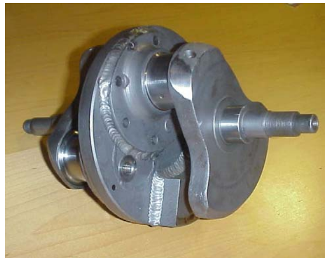
Figure 5 – Norton crank with counterweights and sludge trap plugs before balancing and nitriding.
