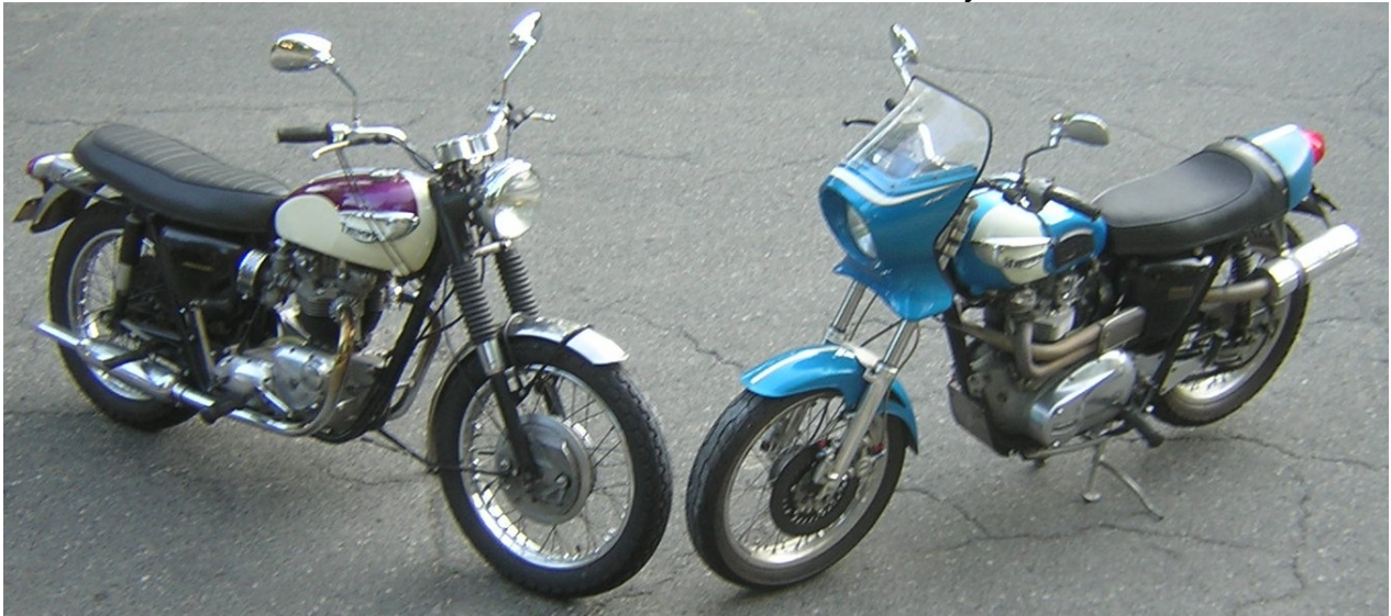
Figure 15 – The original offset-crank Triumph and the latest version with lighter crank; can you see anything different? The 1967 Triumph Bonneville is 650cc with 9:1 pistons, stock exhausts and a Megacycle 510 grind cam. This bike out-accelerates the 1970 750cc single-carb that has 8.4:1 pistons and the same 510 grind cam. The 1970 bike uses a 60% balance factor while the 1967 uses 55%. The 1970 is smoother, and has a higher top speed but the 1967 accelerates faster and is smoother above 5000 RPM. Cruising at 60 mph in 3 rd gear, or a four-speed gearbox, is pleasant where normally a twin rider is hurrying into top gear at that speed.
