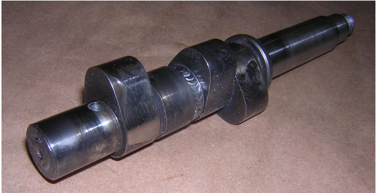
Figure 12 – 67-357 BSA A10 cam, showing weld at one end where centre pin was welded that connects to other half of cam. All welding is done in heavy heat-sink fixture as heat control while welding between lobes is critical. Note hole in cam near left end for indexing fixture.
