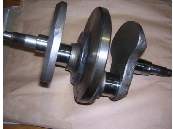
Figure 10 – Norton crank before balance weights added. It will be about 19 pounds.
