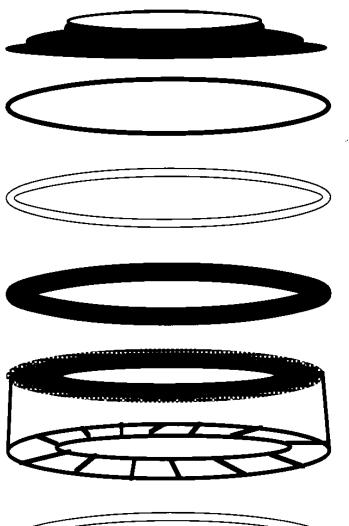
**Dust Wiper-** Generally it is above snap ring. (May be below snap ring on some bikes). Some bikes have dust wipers above and below snap ring.
